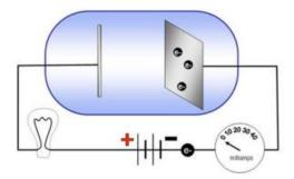
Experiments were performed in **evacuated glass tubes**. The electrons ejected from the surface are called **photoelectrons**. They are the same as electrons in every way.
